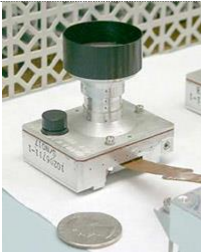
IDC (Instrument Deployment Camera) Crédit image NASA/JPL
